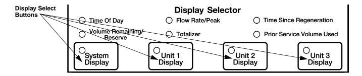
Up To Eight Displays May Be Viewed On The VFD By Pushing The Desired Unit's Display Select Button
